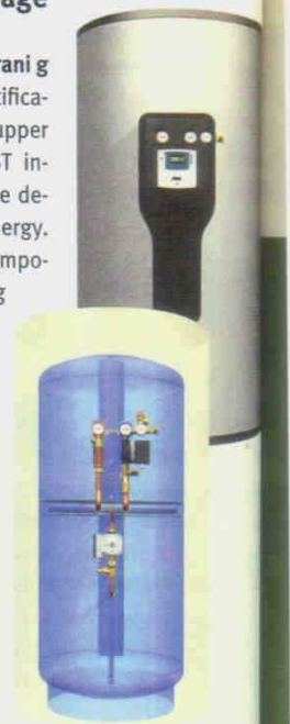
In the stratified storage tank by marani g the stand-by unit and the storage unit are kept apart by a layer separator. Photo: marani g
